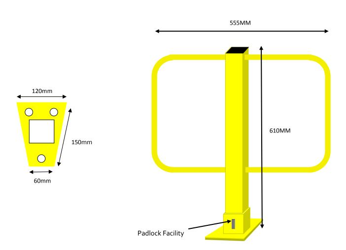
Our SB28 economy post is manufactured with wings in order to alleviate parking between posts. Also fitted with a hinged padlock facility this allows the post to be locked in the upright position and folded down when required.
